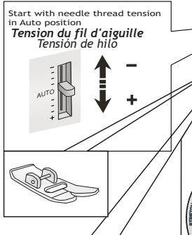
Start with needle thread tension in Auto position
